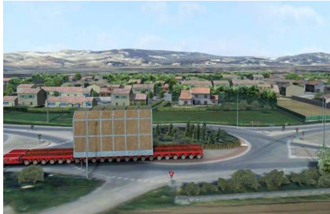
Heavy Component on Road (TF Coils, VV Sectors, & PF1 Coil)
